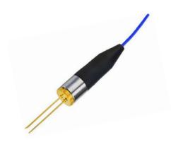
The FPF series fiber-coupled laser diodes are designed with a GaAs quantum well structure integrated with a grating configuration. These diodes feature a built-in photodiode for precise monitoring and feedback control of the laser's output power. Housed in standard TO packages, these diodes are pigtailed to a 1-meter long single-mode fiber terminated with an FC/APC connector. Each unit undergoes rigorous testing prior to shipment to ensure reliability.
